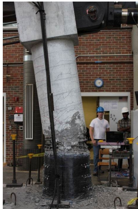
Figure 2.13 Experimental Test B: photo at peak displacement (Rutledge 2012)
